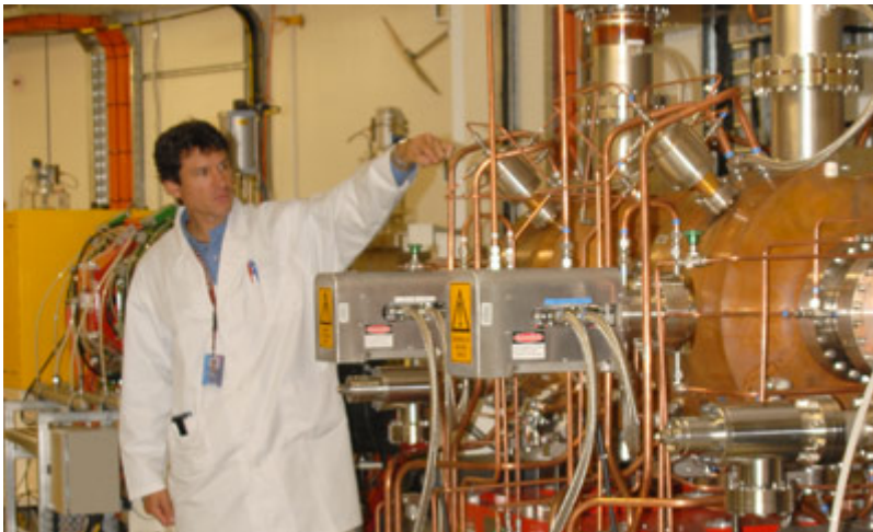
Mark Boland in the storage ring tunnel with two of the four RF cavities
