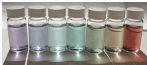
Almost all the colours of the rainbow: gold nanorods in solution, with aspect ratios increasing from left to right (photo: Jonathan Edgar, University of Technology Sydney)
