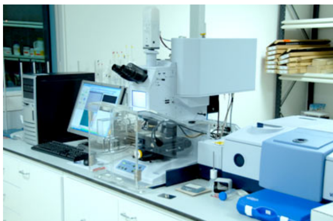
The Hyperion 3000 Infrared Microscope in the synchrotron's chemistry laboratory. (Photo: Mark Tobin)
