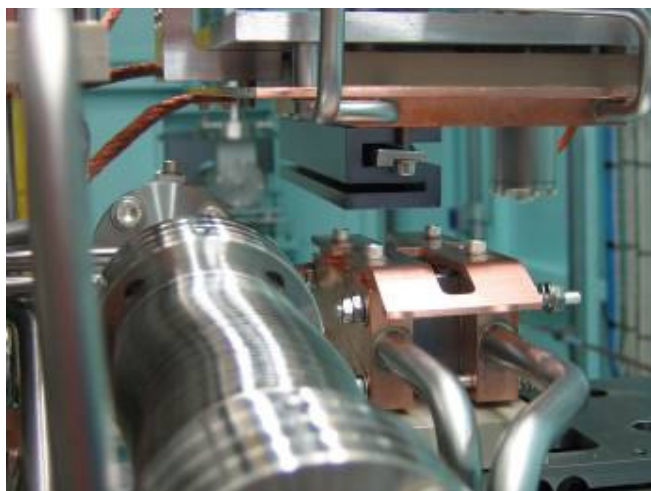
The silicon-111 crystals in the SAXS/WAXS monochromator, which select the required wavelength and help steer the beam
