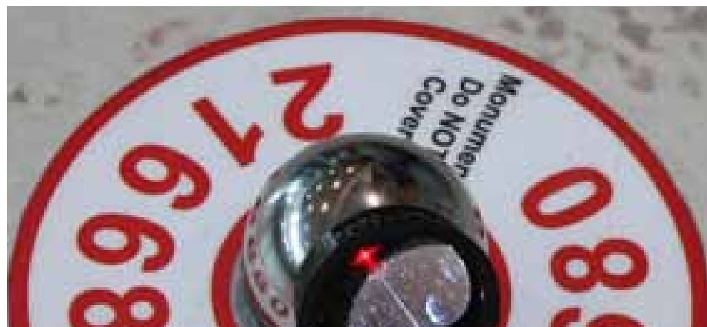
Engineers recently re-measured the precise position of 324 network points like this one
