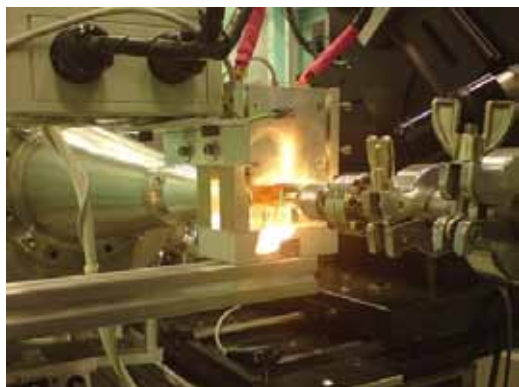
Photo of user-supplied sample cell on SAXS beamline, by Bridget Ingham
