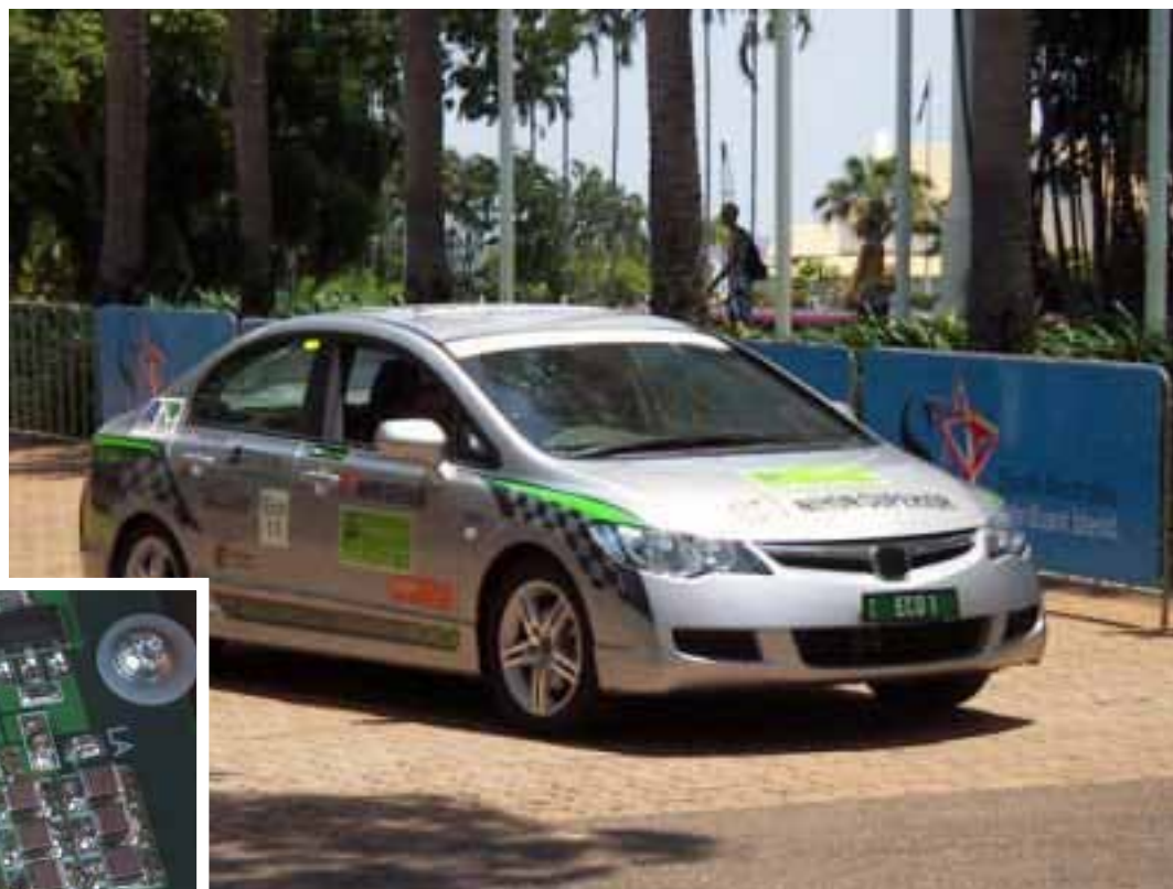
The battery controller circuit board for electric vehicle 'Deep Green Research EV' in the Global Green Challenge from Darwin to Adelaide in October 2009 was soldered with SN100C, a tin-copper-nickel solder alloy that has been the focus of much of Kazuhiro Nogita's research.
