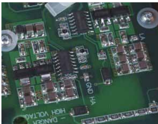
The battery controller circuit board for electric vehicle 'Deep Green Research EV' in the Global Green Challenge from Darwin to Adelaide in October 2009 was soldered with SN100C, a tin-copper-nickel solder alloy that has been the focus of much of Kazuhiro Nogita's research.
