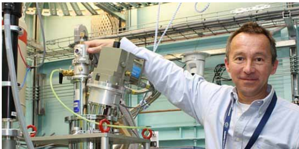
ANU's ion implantation facility is being used to produce doped silicon samples for synchrotron analysis.
