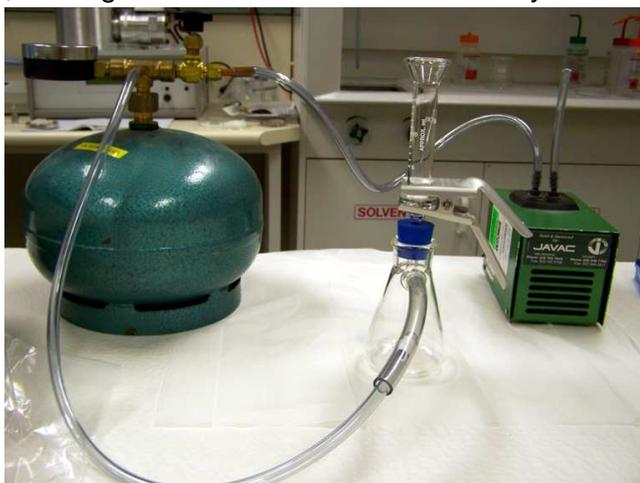
5. Take the solution out of the ultrasonic bath and pour it on the funnel until it is almost full. Then turn on the vacuum pump to suck the liquid through the filter. Particles
